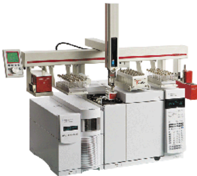
Figure 1. GERSTEL MPS 2 with DHS on an Agilent Technologies 7890 GC.
