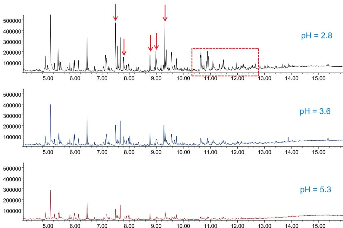
**Figure 5.** Blank chromatograms of EG-Silicone Twisters after water sample extractions at different pH values and subsequent conditioning. The arrows and dashed lines show the polyglycol peaks that increase in size with decreasing pH value.
