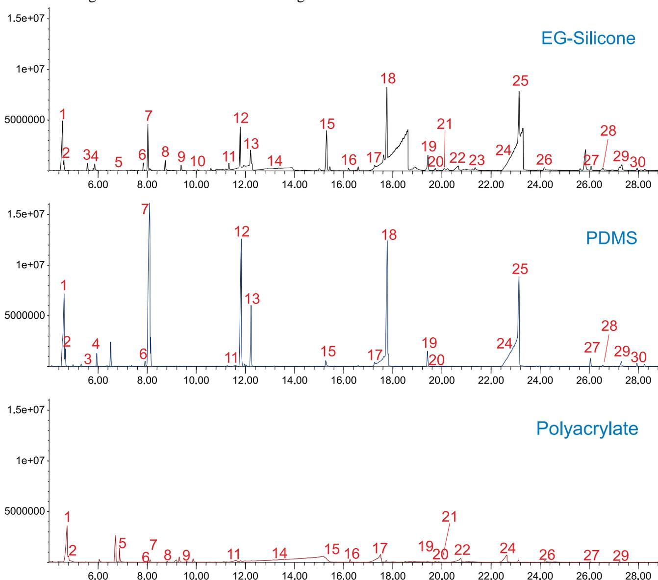
**Figure 7.** Sauvignon Blanc chromatogram profiles obtained from EG-Silicone-, PDMS- and PA Twister extractions of 5 mL samples for one hour at 1000 rpm, non-polar column separation.
