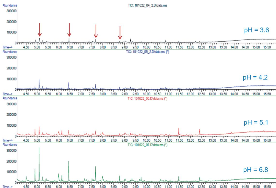
**Figure 4.** Blank chromatograms of EG-Silicone Twisters after wine extraction at different pH values and subsequent conditioning. The arrows indicate the siloxane peaks, which increase in size with increasing pH value.
