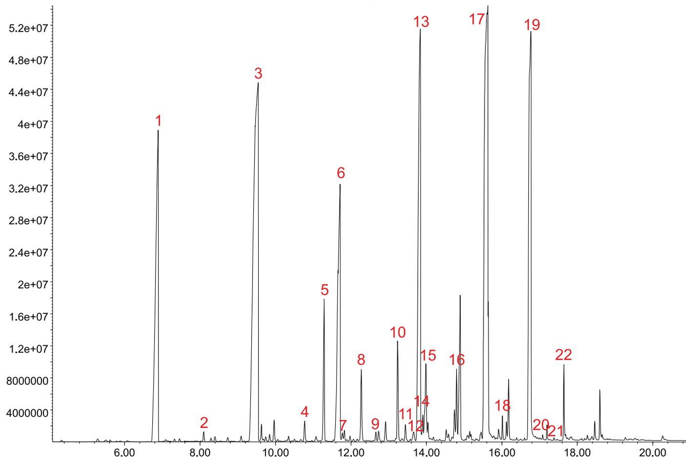
**Figure 2.** SBSE-TD-GC/MS chromatogram, polar column separation, resulting from an EG-Silicone Twister extraction of a 5 mL whisky sample diluted 1:1 with water (20 % EtOH v/v). Sample extracted for 1 hour at room temperature and 1000 rpm.
