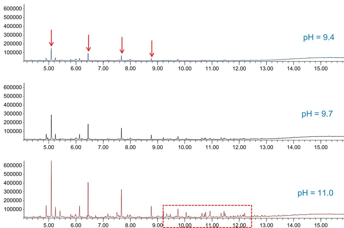
**Figure 6.** Blank chromatograms of EG-Silicone Twisters after water sample extractions at different pH values and subsequent conditioning. The arrows and dashed lines show the siloxane peaks that increase in size with increasing pH value.
