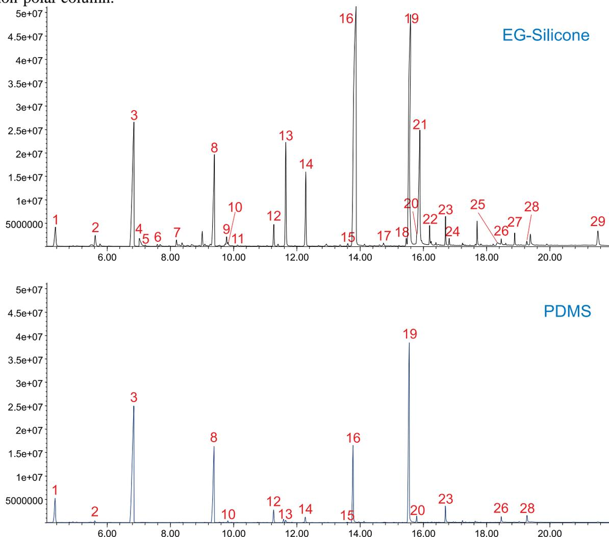
**Figure 8.** Sauvignon blanc chromatogram profiles obtained from EG-Silicone- and PDMS Twister extractions of 5 mL samples for one hour at 1000 rpm, polar column separation.
