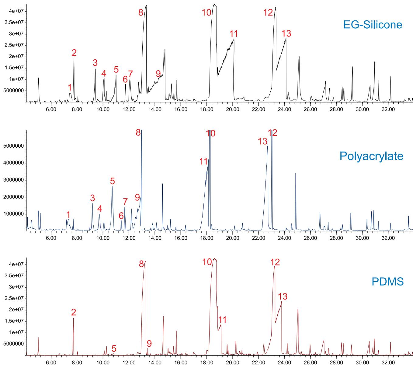
**Figure 1.** Whisky extraction chromatograms obtained using EG-Silicone, Acrylate and PDMS Twisters, non-polar column separation. 5 mL whisky sample (20 % EtOH (v/v), 1:1 dilution with water), 1000 rpm for 1 hour at room temperature. Peak identification: 1. Phenol; 2. C6 Acid ethyl ester; 3. o-Cresol; 4. p-Cresol; 5. Phenethyl alcohol; 6. o-Ethylphenol; 7. 2,4- Xylenol; 8. C8 Acid ethyl ester; 9. C8 Acid; 10. C10 Acid ethyl ester; 11. C10 Acid; 12. C12 Acid ethyl ester; 13. C12 Acid.
