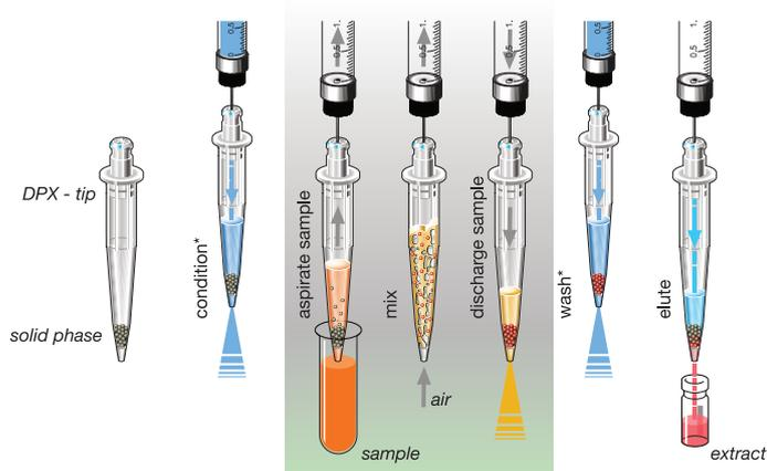
**Figure 1.** Graphical representation of the DPX extraction process.
